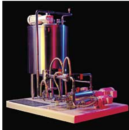
Photograph 1: SeedMaster crystallisation unit for the production of the cocoa butter crystal suspension.
